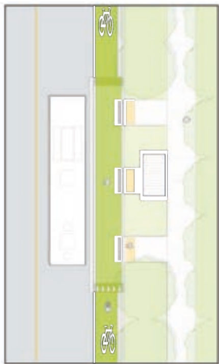
FIGURE 5.25 Raised Bike Lane at Transit Stop
