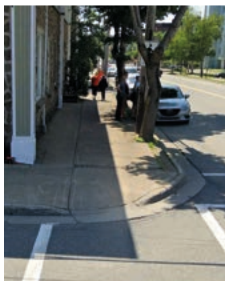
FIGURE 5.15 Apron Driveway Treatment for Separated Bike Lane
