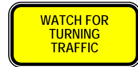
TURNING TRAFFIC TAB SIGN 450 mm x 225 mm Required mounted below Trail Crossing Side Street Sign
