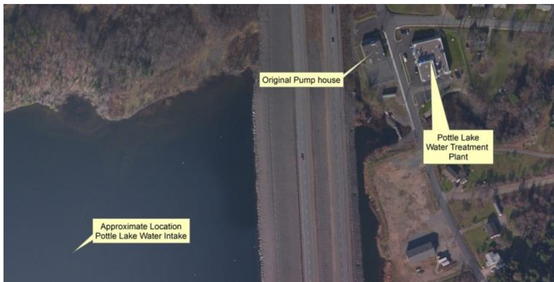
Figure 2. Intake left of Highway 125; pump house and treatment plant on the right.
